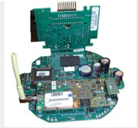
Smart enough? This image shows the interior of a smart grid meter tested by Mike Davis of IOActive. Credit: Mike Davis
